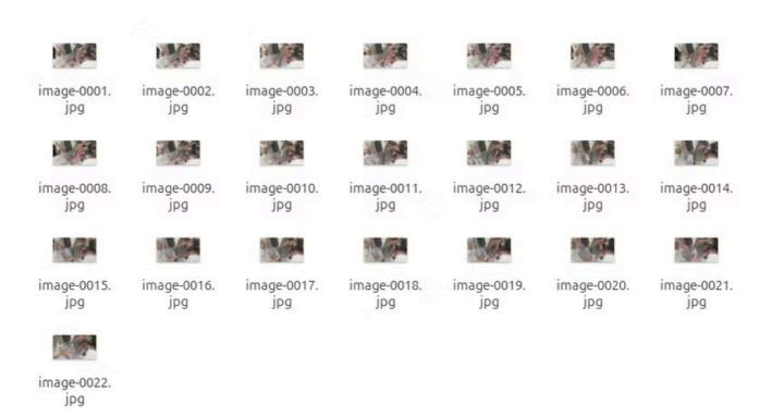
Here, option "-r 1" sets the capture rate to one picture per second. It extracts one frame from each second of the video. You can adjust this number to capture
